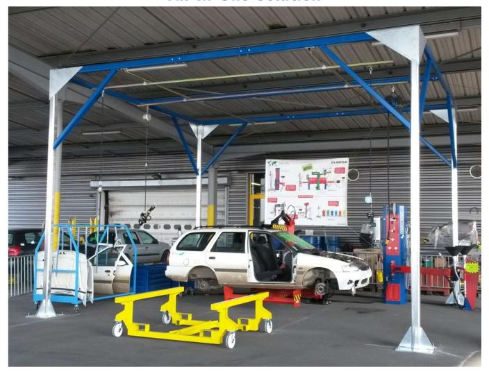
This solution is the first complete system for ELV depollution and dismantling which now can be performed on a new special TiltLift by one person independently.
