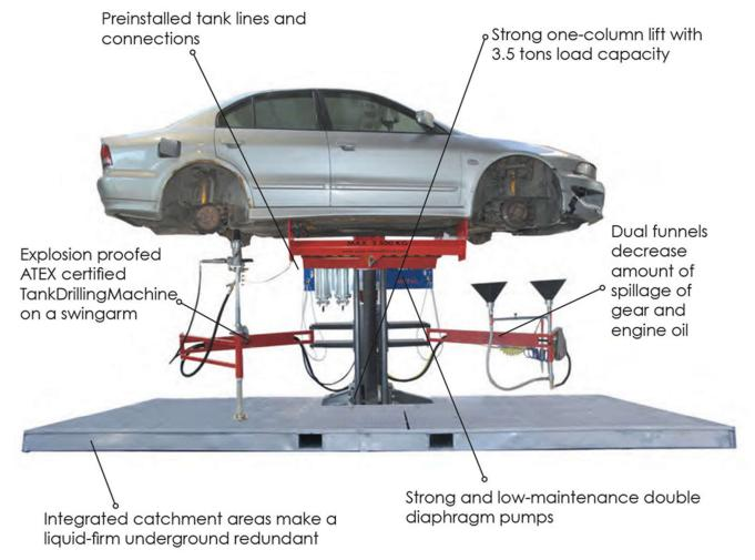
The MDS2 Plattform DrainLift is the ideal combination of a single hydraulic lift with the tried and tested drainage system, situated on a mobile platform. Also simple dismantling work can be done on it hasslefree.
