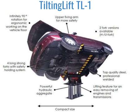
It is easy to place a car into the system. Secured by a hydraulic safety arm on the top, the car is ready to turn 70° in order to help a worker to stand upright and work on the car bottom easily.
