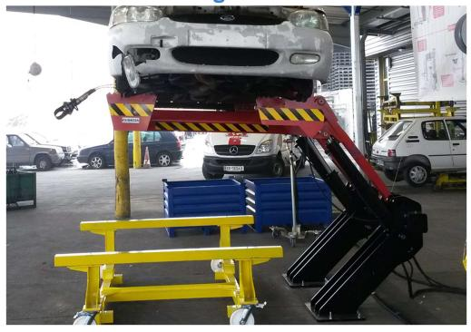
It is easy to place a car into the system. Secured by a hydraulic safety arm on the top, the car is ready to turn 70° in order to help a worker to stand upright and work on the car bottom easily. Furthermore it is possible to lift the car up to 1850 mm.
